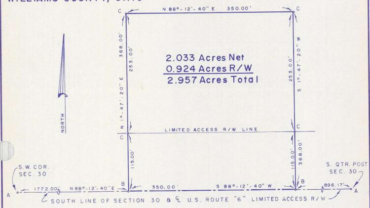
ALL DIMENSIONS ARE SHOWN IN FEET AND DECIMAL PARTS THEREOF. DIMENSIONS ON CURVES ARE CHORD MEASURMENTS. THIS SURVEY HAS BEEN FILED IN VOLUME 10K PAGE 257 OF THE WILLIAMS COUNTY RECORD OF SURVEYS, COURTHOUSE, BRYAN, OHIO.
